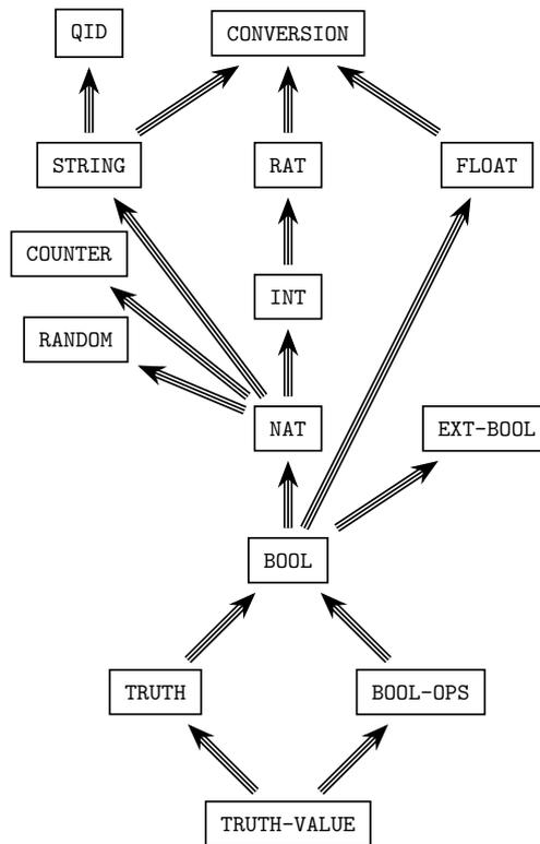
Figure 8.1: Importation (protecting) graph of predefined modules
